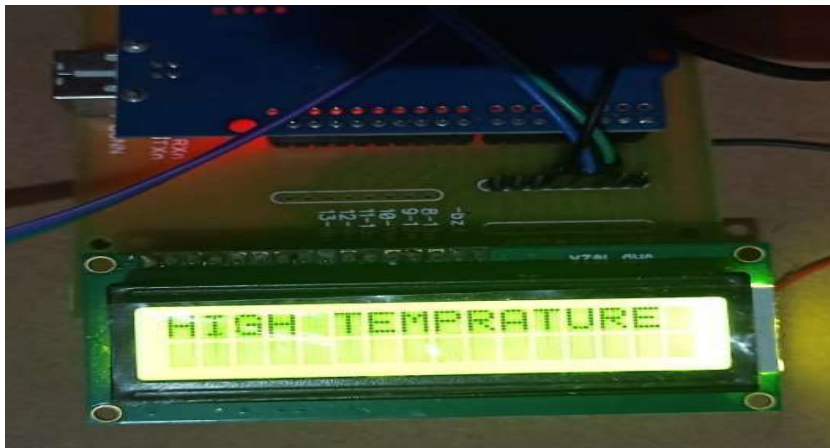
Fig 3.2 Displayed on LCD as HIGH TEMPERATURE (td>35)
